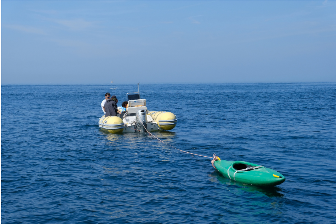
Figure 1.4: Boatbot towing a kayak and a magnetometer, Bay of Brest, July 2018.
